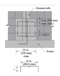
If continuous horizontal reinforcement is not otherwise provided within the end 8 in. (203 mm) of each end of the splice, confinement requirements may be satisfied by providing hooked reinforcement as detailed here. See Tables 4a through 4d for  $l_i$  minimum length requirements. Hook extensions are permitted to overlap.
