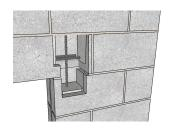
**Third**, the masonry wall CJ's should be located away from openings. Masonry lintels create an integral joint with vertical jamb reinforcement. This leads to a more robust design that has many analysis and design benefits including arching action and fully developed lintel
