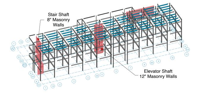
Contractor: The masonry stair and elevator shaft walls in the above project are being used by the architect/engineer design team as impact resistant, durable, and fire resistant walls. The walls are also resisting gravity floor and roof loads. Are there other other ways that the masonry walls can be utilized?
